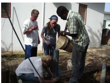
Dr. Randy Lewis watches as students test the permeability of sand.
